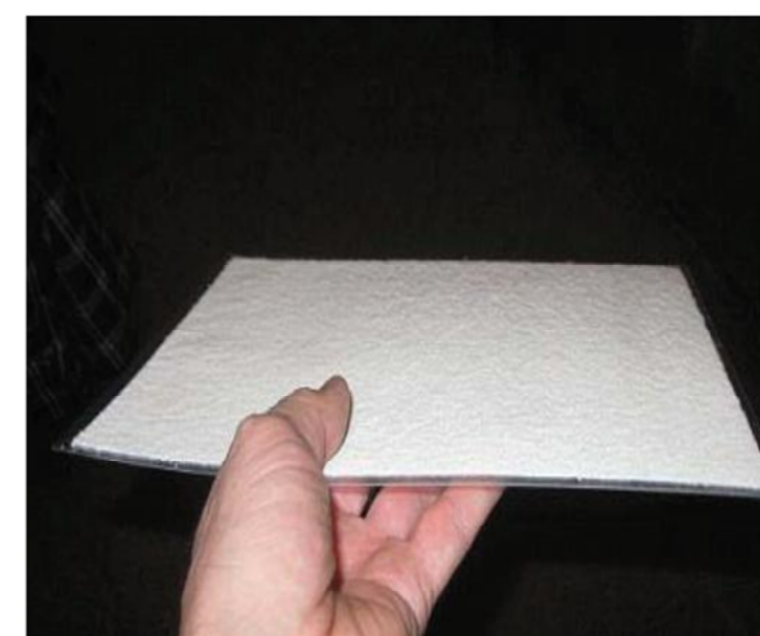
Left – a sheet of ZnS(Ag)+ 6 LiF scintillator, right – the 6 Li(n,t) 4 He total cross section
