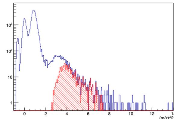
Figure 3. The squared mass-to-charge distribution for albedo particles in energy range for tritium from 50 to 63 MeV/nucleon. No selection applied for blue distribution and energy loss cuts applied to the red one.
