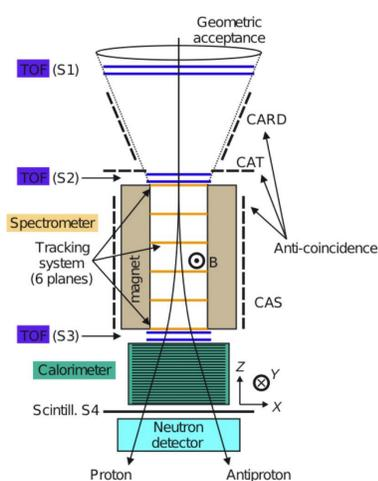
Fig. 1. Scheme of PAMELA instrument.
