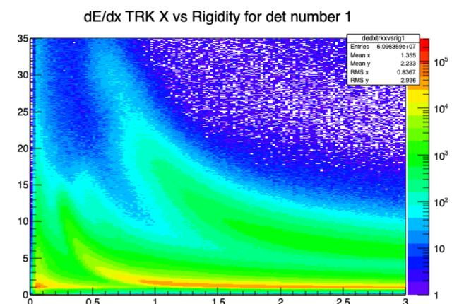
Figure 2. The dependence of energy losses in the second X-view plane of the tracker on reconstructed particle rigidity.
