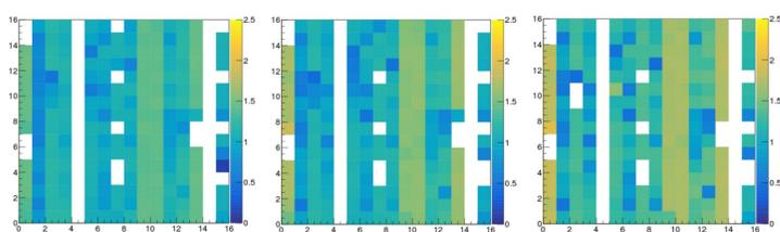
Calibration of PMTs and comparison to pre-flight measurements. Relative PMT gain calibration was done by analyzing background events and is presented here for 2 statistically independent subsets of data (left and center). Pre-flight measurements (right) are shown with 2 PMT modules that later stopped working turned off for comparison.
