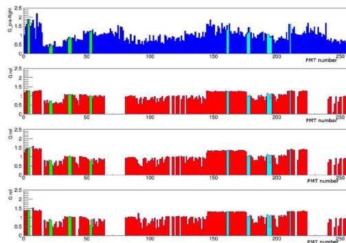
Relative PMT gain coefficients for all 256 channels according to pre-flight measurements (top) and reconstructed from background data for first 3 half-years of operation. The light color corresponds to the PMT of the selected events
