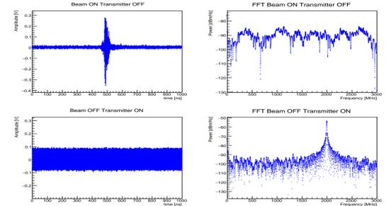
Figure 5: Example of Beam-only event and transmitter-only events with their FFT spectra.
