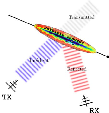
Figure 3: Schematic representation of the radio reflection from a particle cascade.
