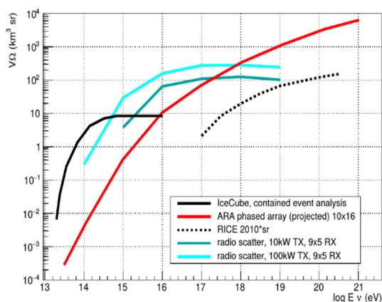
Figure 2: Calculated target effective volume for UHE neutrino detectors. The radar technique has the best projected sensitivity in the  $10^{15}$ – $10^{18}$  eV range. Figure taken from [3].
