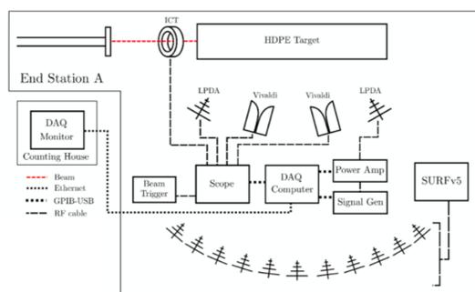
Figure 4: Experimental setup from Run 2.
