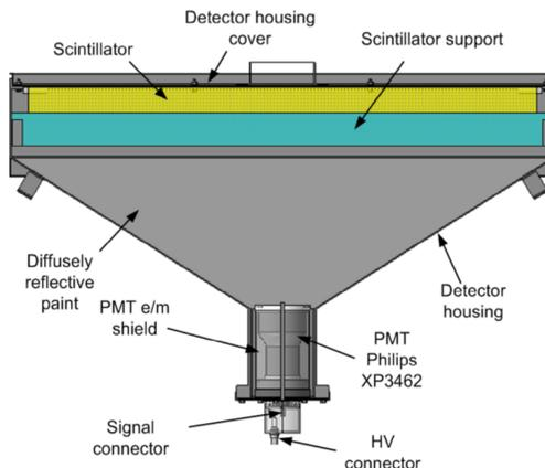
Construction of the scintillation counter
