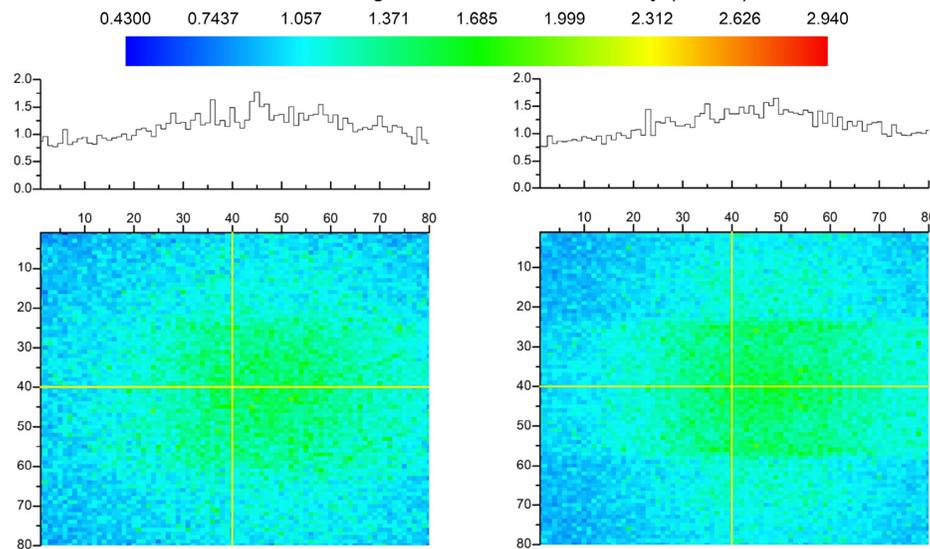
The matrices of the mean charge of the counter response to passage of a single muon
