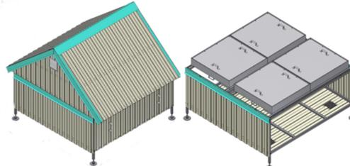
Detector station housing (left) and layout of counters inside the DS housing (right)
