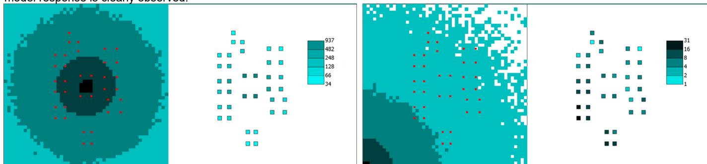
The simulation of the NEVOD-EAS array response to the passage of extensive air shower: the density of secondary particles (left) and DS responses in terms of vertical equivalent muon (right)
