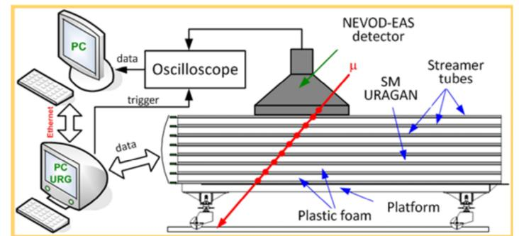
Experimental facility for studying of the light collection non-uniformity of the NEVOD-EAS scintillation counters
