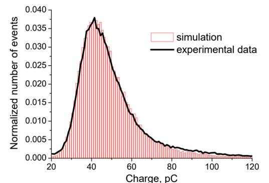
Charge of the counter response to passage of a single muon
