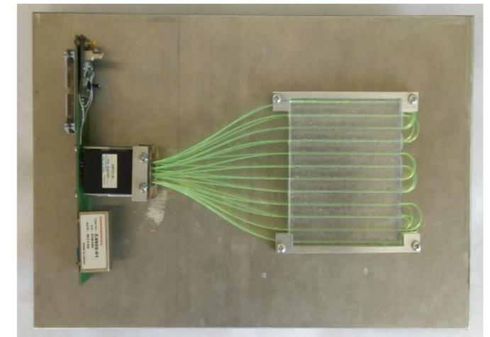
Scintillation detector plane of the OLVE-HERO prototype,
