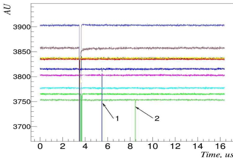
Figure 5. Example of time dependences for the single event amplitudes with neutron picks (1 and 2).
