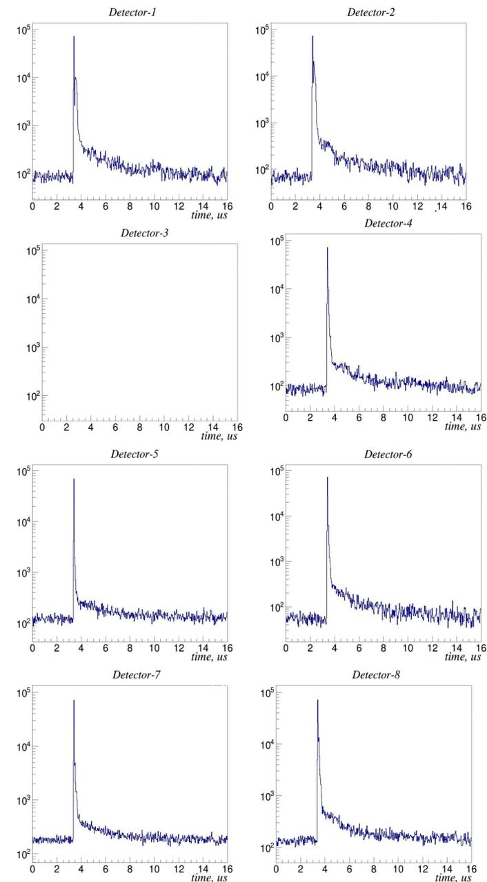
Figure 6. The time dependence of the BS neutron signals after the prototype shifts. Odd numbers of detectors are upstream of beam, even numbers are downstream of beam.
