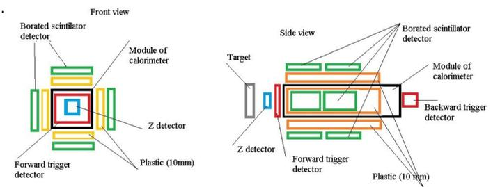
Fig. 1. Schematic view of the OLVE-HERO prototype on the SPS test beam at CERN
