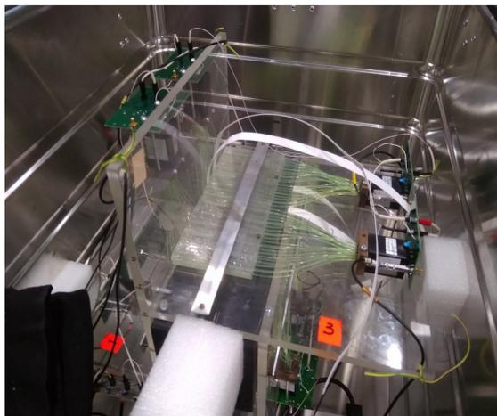
Figure 2. The borated scintillator planes OLVE-HERO inside of light-tight metal container
