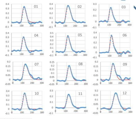
Figure 5. Gamma distribution approximation to Wiener deconvolution results in 12 channels. Horizontal axes:  $t$ , ns; vertical axes:  $f_{out}(t)$  in arbitrary units. Reconstructed input signals are indicated by points; gamma distribution fits are shown by solid curves
