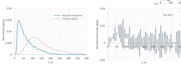
Figure 4. An example of reconstruction of the noisy signal. Left panel: Impulse response and the measured output signal of the system; Right panel: deconvolved input signal.
