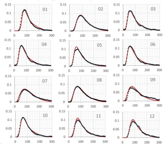
Figure 8. Measured and modeled output signals with fitted gamma distribution as input signals in 12 channels. Horizontal axes:  $t$ , ns; vertical axes:  $f_{out}(t)$  in arbitrary units. Experimental data are indicated by points. The convolution of the impulse response and trial gamma distribution as an input signal is shown by solid curves in each channel
