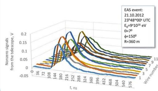
Figure 2. Output signals of WFOV Cherenkov telescope's data acquisition system from EAS event.
