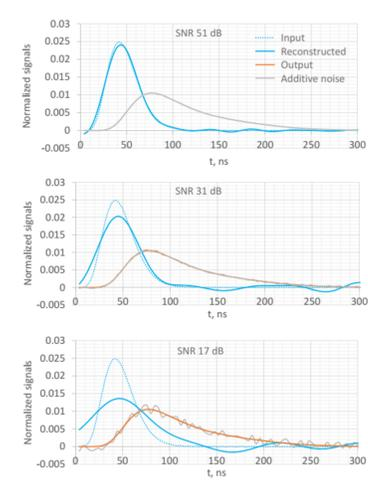
Figure 6. Wiener deconvolution of a noisy signal in a toy model.
