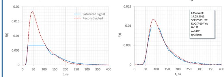
Figure 9. Reconstruction of two saturated output signals from EAS event denoted in the right panel
