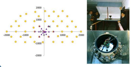
Figure 1. The map of surface stations of the Yakutsk array, distances in meters. Circles indicate stations with scintillation counters producing T500 trigger; triangles show the central cluster of Cherenkov radiation detectors producing an additional trigger. A cross marks the position of the telescope shown at bottom right. A scintillation counter is shown at the upper right
