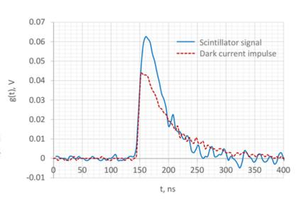
Figure 3. Impulse response of the system to short input signals.
