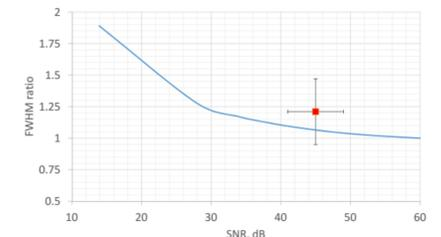
Figure 7. The ratio of durations of Wiener deconvolution and input signals vs SNR in a toy model (solid curve). The red square indicates the ratio of estimated signal durations of the telescope, as described in Section
