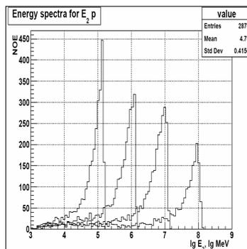
Fig.3. Reconstructed protons energy distributions for discrete values of the primary energy
