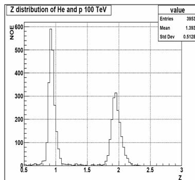
Fig.2. The simulated charge distribution for high energy protons and helium nuclei
