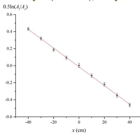
Fig. 5. Logarithmic ratio of amplitude of signals from the left and right ends of prototype detector. The inverse slope of the linear fit indicates the attenuation length  $\lambda = 91 \pm 1$  cm of scintillation light in the scintillator strip
