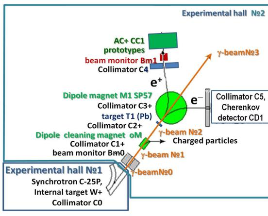
Fig. 2. The beam formation setup and apparatus installation at C-25P synchrotron "PAKHRA"
