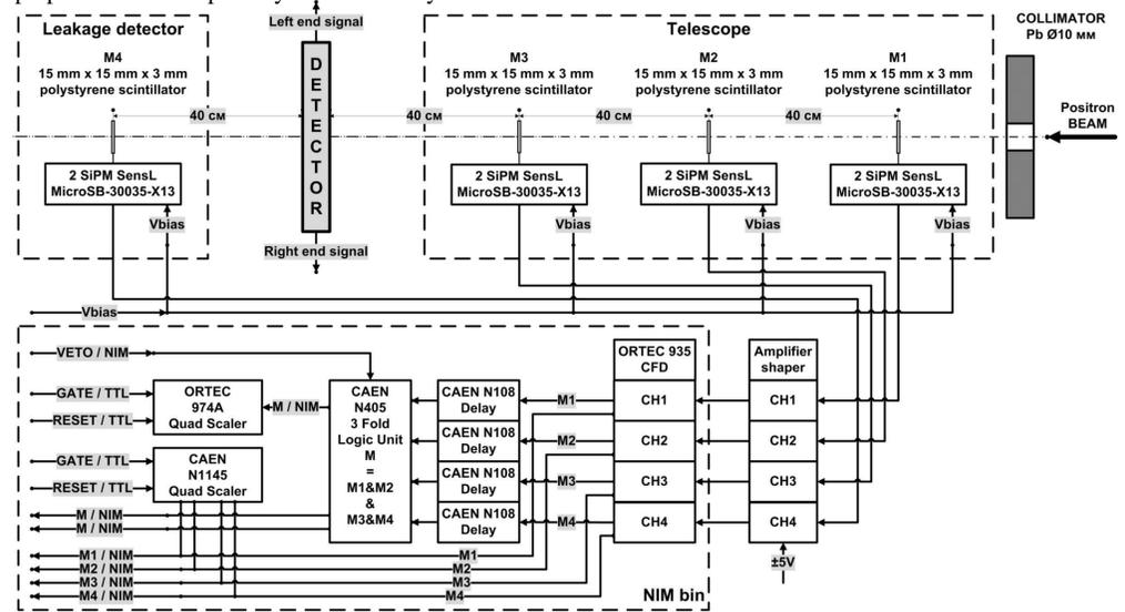
Fig. 4. Experimental setup, including beam monitor. The dash-dotted line represents the beam line
