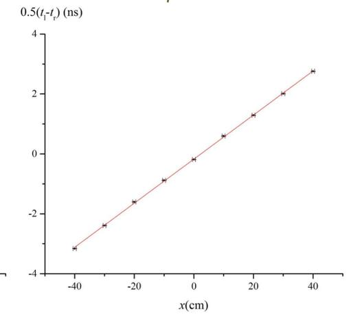
Fig. 6. Straight line fit to the semi difference of time of scintillation light arriving at strip ends at different beam positions relative to the detector centre. The inverse slope of the fit gives the effective scintillation light velocity  $13.1 \pm 0.1$  cm/ns in the scintillator strip
