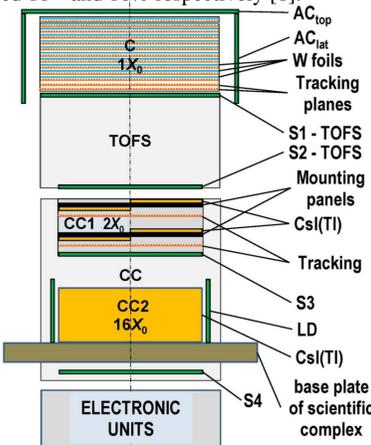
Fig. 1. The sketch of the GAMMA-400 gamma-ray telescope
