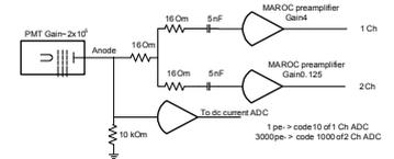
To expand the dynamic range, two channels of ASIC MAROC3 process signals from the same PMT. Signals from each PMT are transferred to the scheme of current monitoring.
