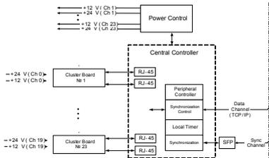
The data acquisition system (DAQ) of the atmospheric Cherenkov telescope camera is modular and consists of 23 identical Cluster board serving the PMT units and the Central unit of the system – the Central Controller. Central Controller provides control of operation of Cluster boards, development of a common trigger, synchronization, data collection from Cluster boards and data storage in the intermediate buffer, data exchange with the Central computer.
