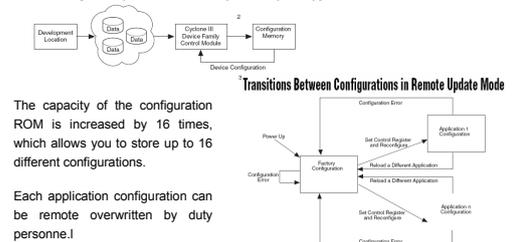
The capacity of the configuration ROM is increased by 16 times, which allows you to store up to 16 different configurations.
