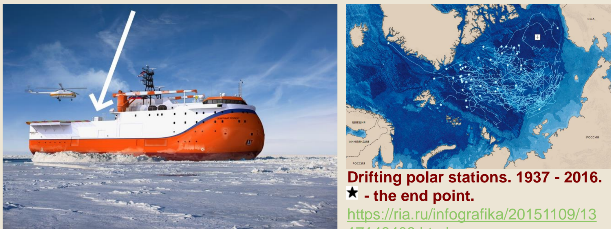
All-season self-propelled platform. Planned date of entry 2020 Arrow - a container of detectors in the stern of the vessel.
