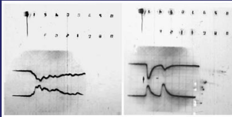
**An example of signal registration by two PMT registering signals from a single scintillation plastic. Observation of the delayed signal by two PMT indicates on the existence of the delayed particles and absents of PMT after – pulses.**
