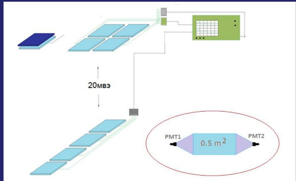
The installation has several scintillation detectors, the signals from which were recorded with help of an analog storage oscilloscope.
