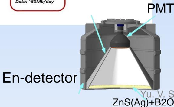
Electron Neutron Detector Array
