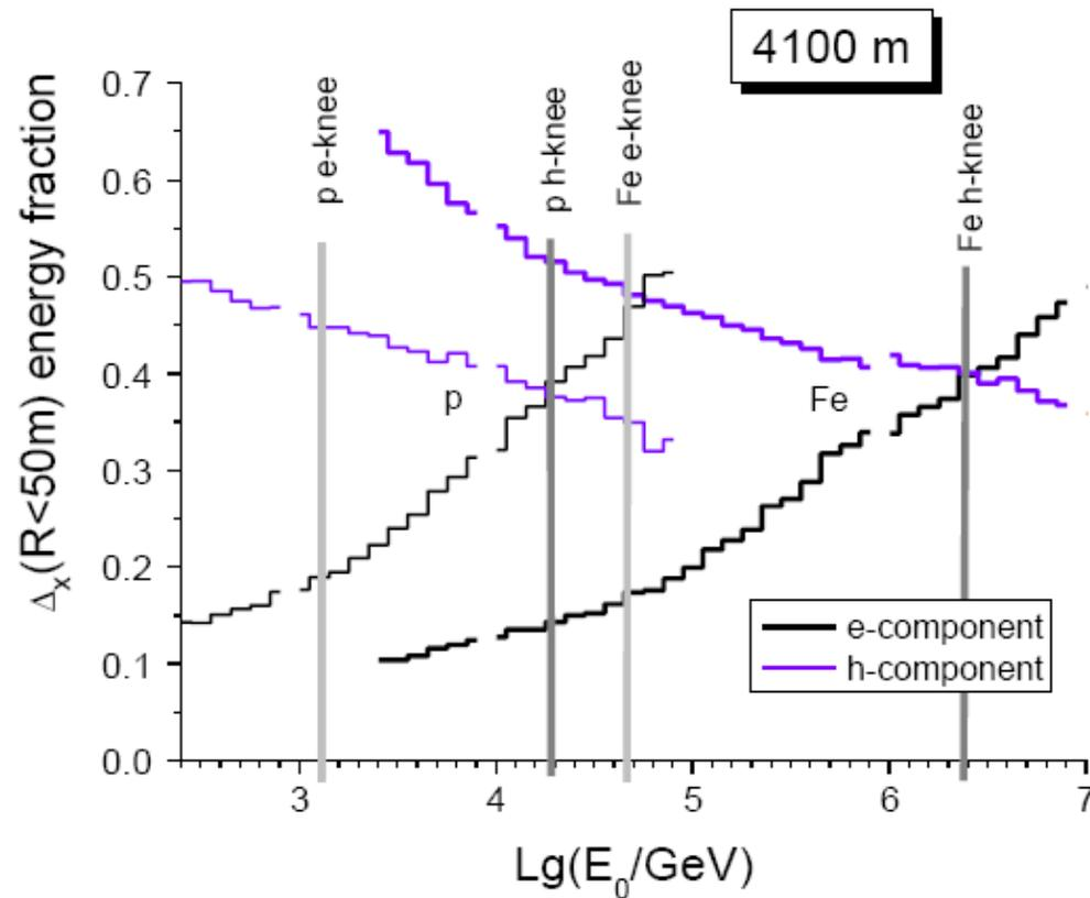
Fig. 1. EAS energy fraction inside a ring of 50 m radius carried by hadronic and electromagnetic components at 4100 m above sea level as a function of primary energy.
