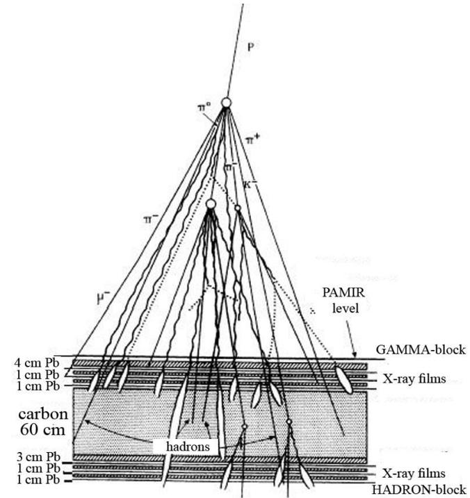
Carbon XREC registers  $\gamma$ -quanta and hadrons formed in the air cascade.
