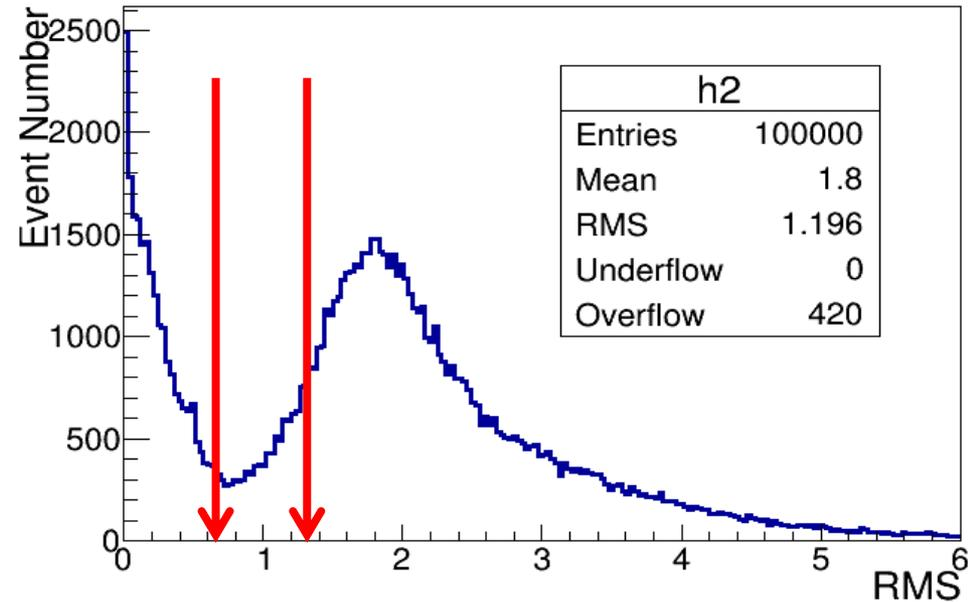
Electron efficiency  $\varepsilon = 0.9$ , proton rejection factor  $f \sim 50$
