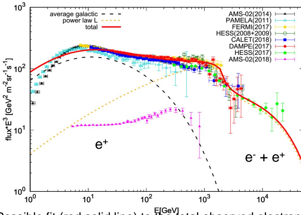
Possible fit (red solid line) to the total observed electron spectrum due to distant sources (black line) and one local continuous fading source (orange dotted line) with  $t/\tau=0.08$
